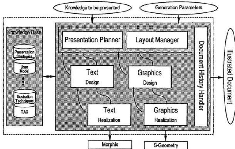
Fig. 2: The Architecture of the WIP System
